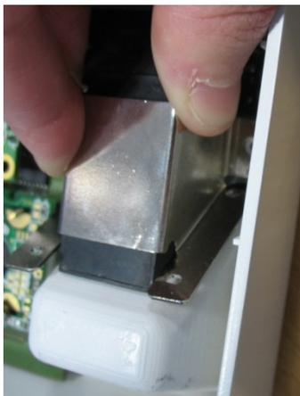
Connect the new sensor by sliding the ribbon into the connector, with the plastic insulating part on the board side, then fold back the black locking tab.
